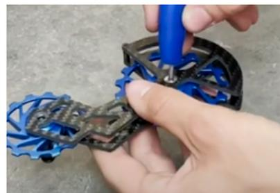
**Unscrew the M4x8 screw by using the 4 mm Allen key.**
