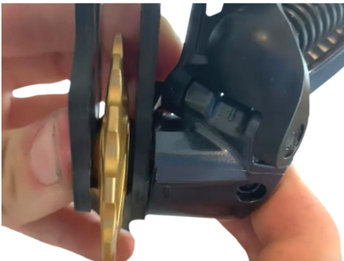
**Keep the cage sunk into the derailleur until screwing the screw back on.**
