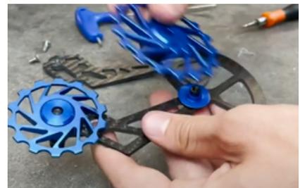
**Put back the carbon back and screw the M4x10 and M4x8 by using the 4 mm Allen key with a little bit of thread-locker to lock the screws.**
