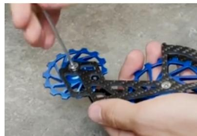
**Unscrew the stopper by using the 2 mm Allen key.**
