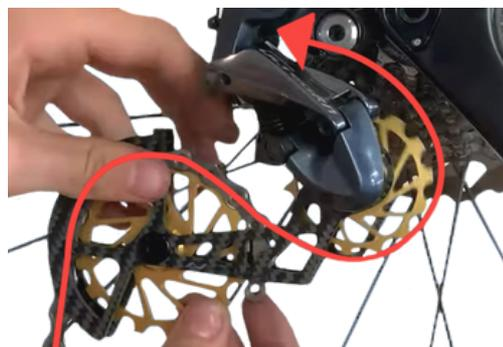
**After the installation, the chain length changes. So it is highly recommended to use a new chain. Visit the link below to watch our video "How To Calculate The Correct Chain Length".**
