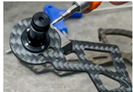
**Once the stopper is well installed, put back the 14T and the 17T pulley wheels as well as the covers.**
